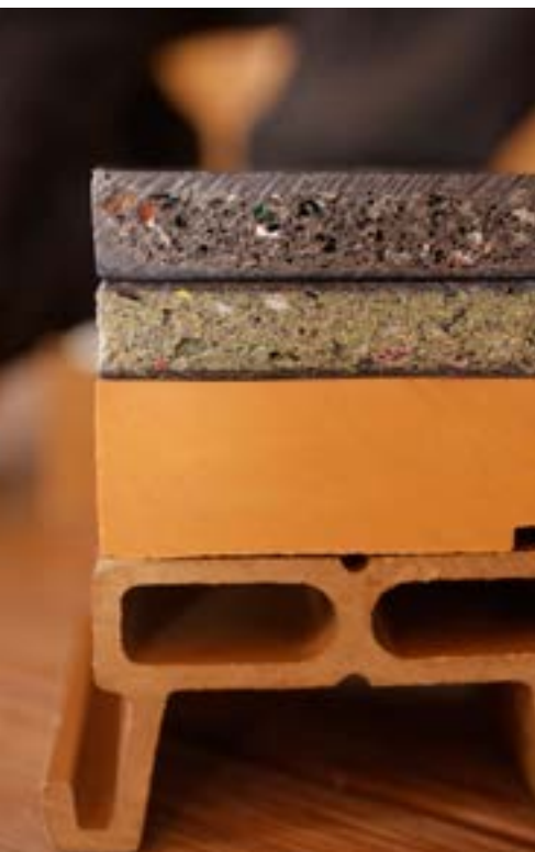
BELOW: Cross-sections of Nev House recycled construction materials. Note the flecks of coloured electronic cable sheathing in the compound.
